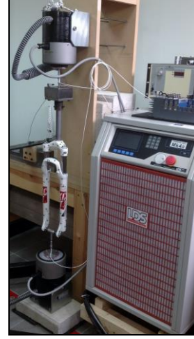
Figure 9: Schematic illustration and experimental arrangement of suspension sub-assembly
