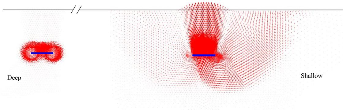
Figure 4. Failure mechanisms for an anchor embedded at  $H/B = 2$  for two different random field realisations.
