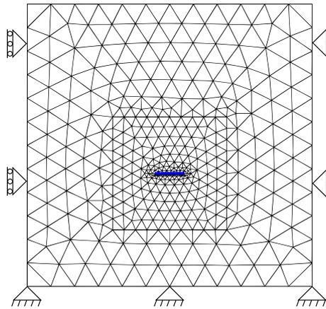
Figure 2. Typical FE mesh ( $H/B = 2$ ).
