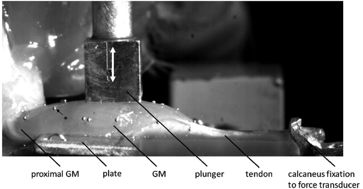
Figure 1: Experimental setup. Transversal load is induced on rat *M. gastrocnemius medialis* (GM) by a plunger which is able to move freely in vertical direction. The small markers on the muscle surface (\*) were used for analyses in another study.
