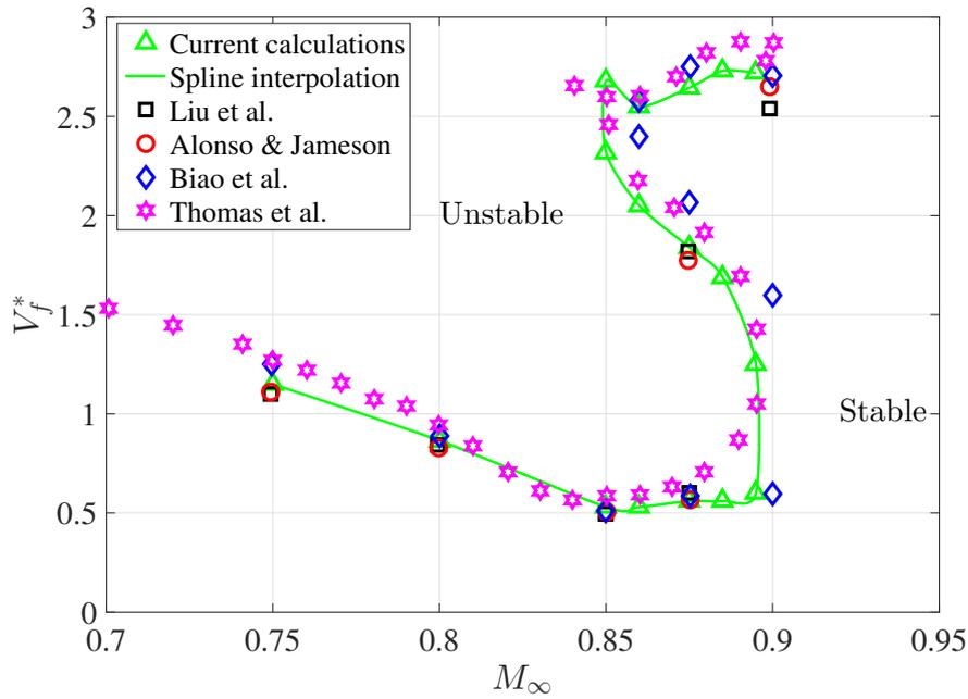
Figure 15: Flutter speed index as a function of the free-stream Mach number. Comparison between current computations and numerical results from the literature.
