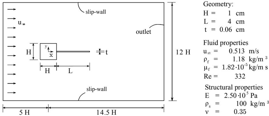
Figure 21: Benchmark for FSI solver with deformable solids.
