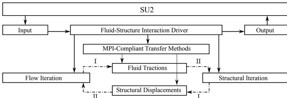
Figure 5: Transfer structure for Fluid-Structure Interaction problems.
