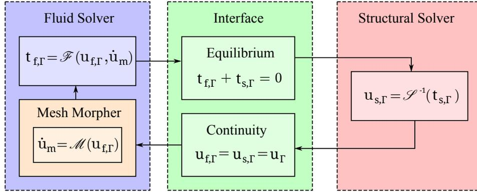
Figure 6: Block Gauss-Seidel subiterations for strong coupling.
