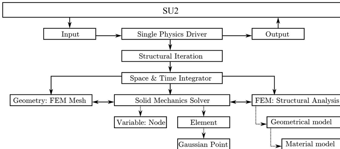
Figure 3: Structure of the Solid Mechanics solver.
