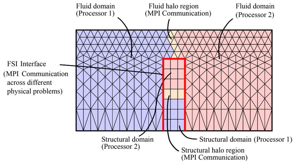
Figure 4: Sample FSI problem run in multiple cores.
