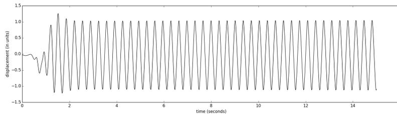
Figure 28: Time history of vertical tip displacements obtained using the python based coupling
