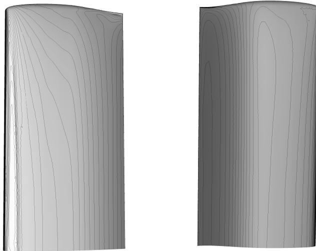
Figure 16: Steady state solution, pressure coefficient distribution over upper and lower wing sides
