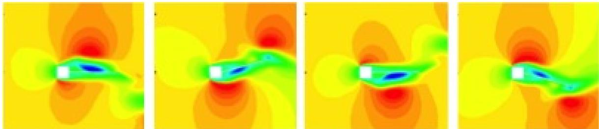
Figure 29: Convective flux contours and structural displacements for the benchmark test cases (using the python based framework) for a full cycle of oscillation. From left to right,  $T=0$ ,  $T=\pi/2$ ,  $T=\pi$ ,  $T=3\pi/2$ .
