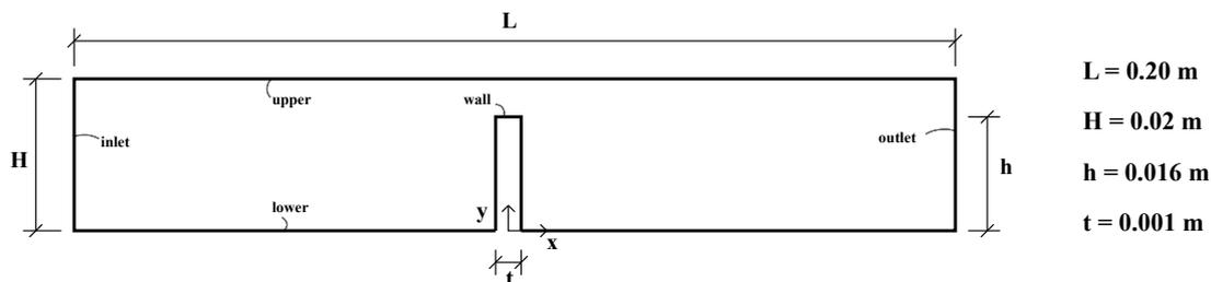
Figure 24: Test case used for interpolation routines.
