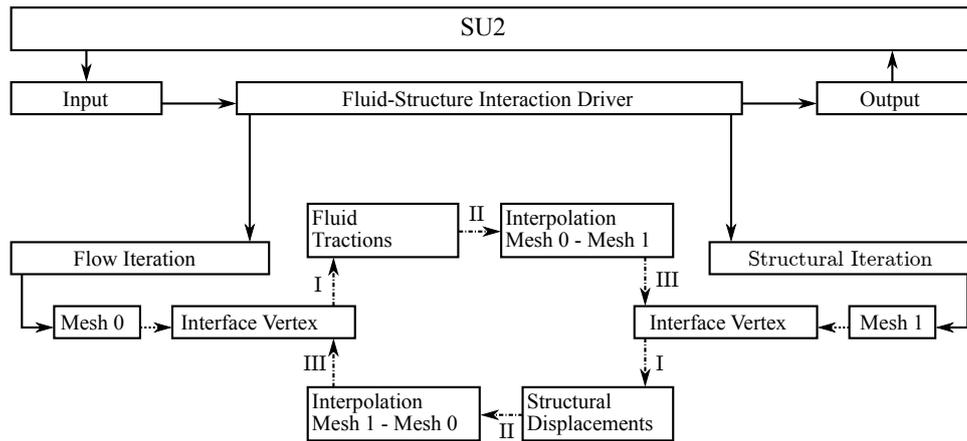
Figure 7: Interpolation structure for Fluid-Structure Interaction problems.
