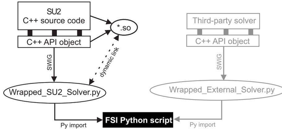
Figure 8: Python wrapping of SU2, from source code to FSI script (black). A symmetric architecture can then be applied to the structural solver (gray).
