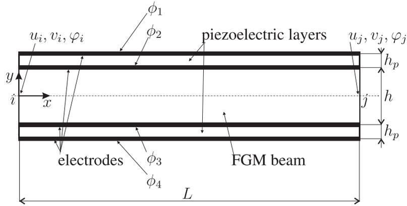
Figure 1: Electric DOF in 2D beam element
