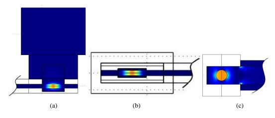
Figure 6: Distribution of the heating rate Q: a) top-view, b) side-view, c) cross-section.
