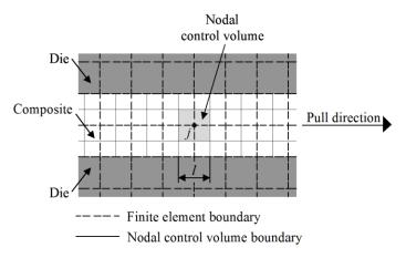
Figure 3: Finite element and nodal control volume meshes.
