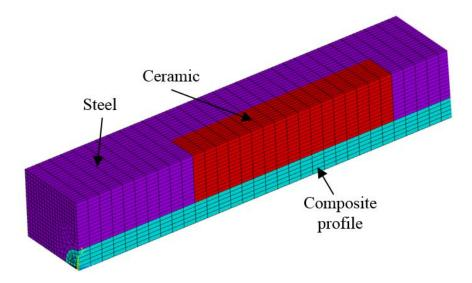
Figure 11: Fragment of the finite element model.
