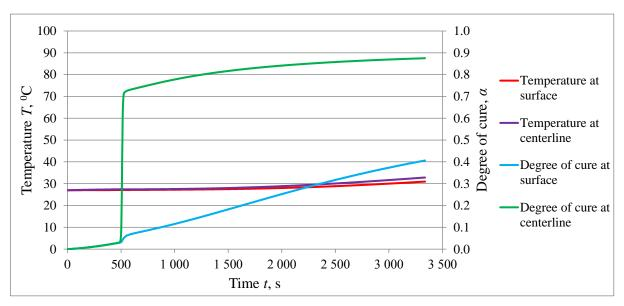
Figure 12: Dependence of temperature and degree of cure in the composite at the die exit on time for room temperature 27°C and pull speed 12 cm/min.
