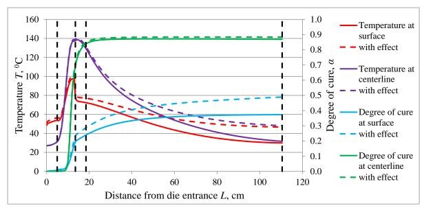
Figure 16: Temperature and degree of cure at the profile centerline and surface taking into account the effect of preheating of steel die.
