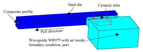
Figure 5: Scheme of the microwave model.
