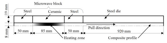
Figure 8: Scheme of the advanced pultrusion die.
