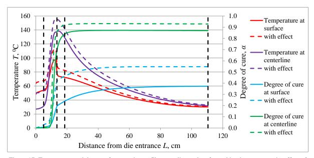
Figure 17: Temperature and degree of cure at the profile centerline and surface taking into account the effect of heating of resin bath.
