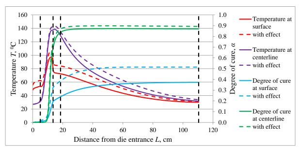
Figure 15: Temperature and degree of cure at the profile centerline and surface taking into account the effect of thermal insulation.
