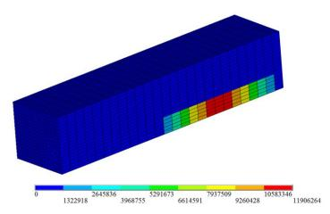
Figure 10: Simulation of the absorption energy in the pultruded profile.
