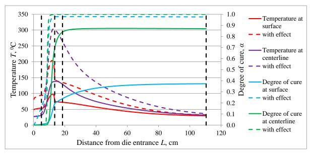
Figure 19: Temperature and degree of cure at the profile centerline and surface with the intensity coefficient of the absorption energy field equals to 2.5 (pull speed: 12 cm/min).
