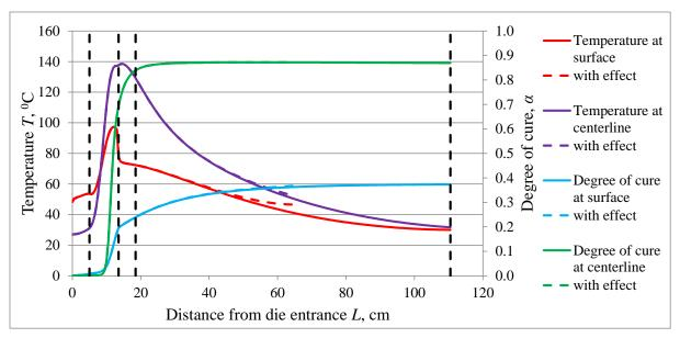
Figure 14: Temperature and degree of cure at the profile centerline and surface taking into account the effect of reduction of steel die length.
