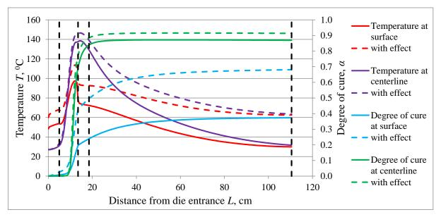
Figure 18: Temperature and degree of cure at the profile centerline and surface taking into account the effects of thermal insulation and preheating of steel die.
