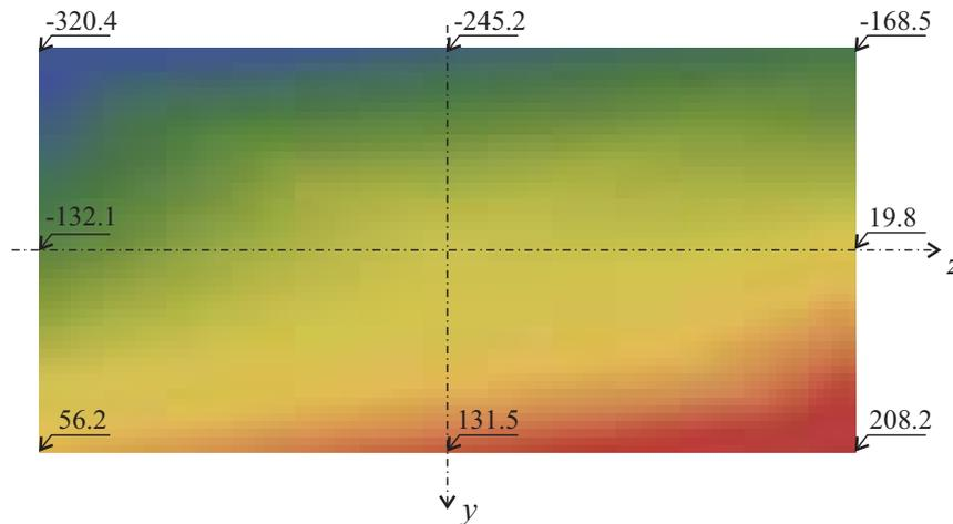
Figure 18: Resultant normal stress  $\sigma(x, y, z)$  [MPa] at position  $x = 0$  calculated by our approach [18].
