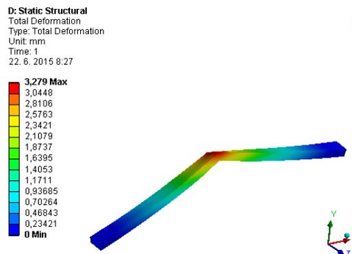
Figure 8: Total deformation of the FGM beam structure.
