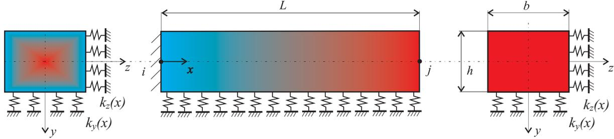
Figure 9: Clamped beam on elastic foundation with spatially varying material properties.
