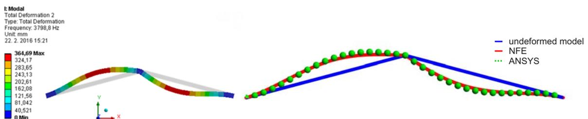
Figure 6: The 2<sup>nd</sup> eigenform of the FGM beam structure displayed by the ANSYS postprocessor and comparison of NFE and ANSYS.
