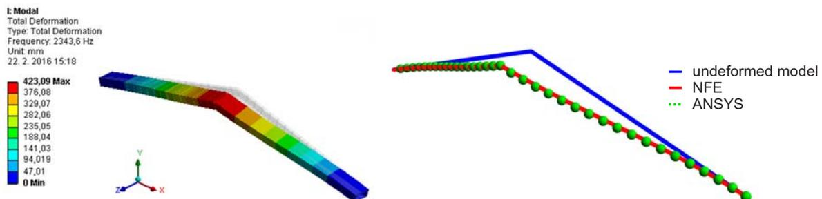
Figure 5: The 1<sup>st</sup> eigenform of the FGM beam structure displayed by the ANSYS postprocessor and comparison of NFE and ANSYS.
