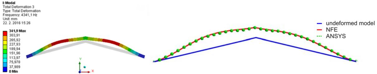
Figure 7: The 3<sup>rd</sup> eigenforms of the FGM beam structure displayed by the ANSYS postprocessor and comparison of NFE and ANSYS.
