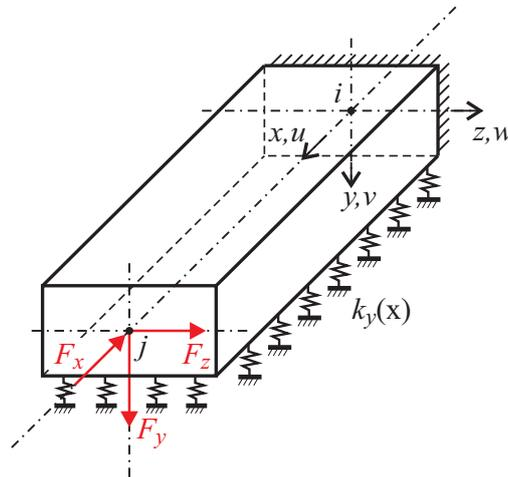
Figure 12: Loaded FGM beam.
