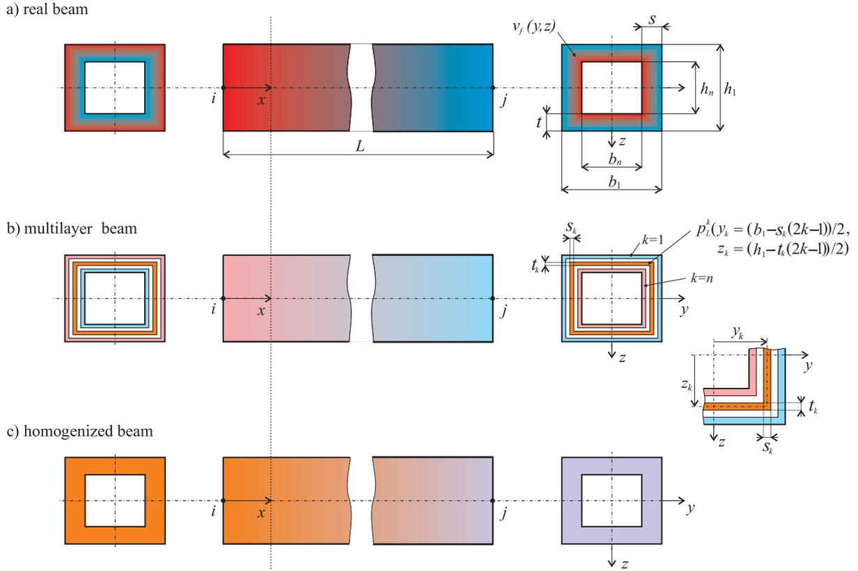
Figure 3: A straight FGM beam of hollow cross-section.
