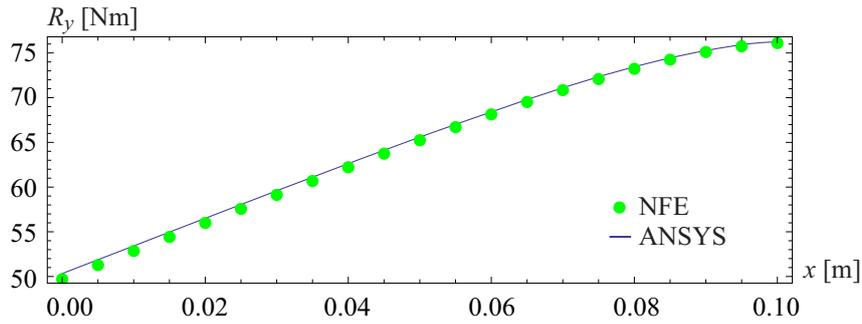
Figure 16: Transversal force in  $y$  – axis (without elastic foundation).
