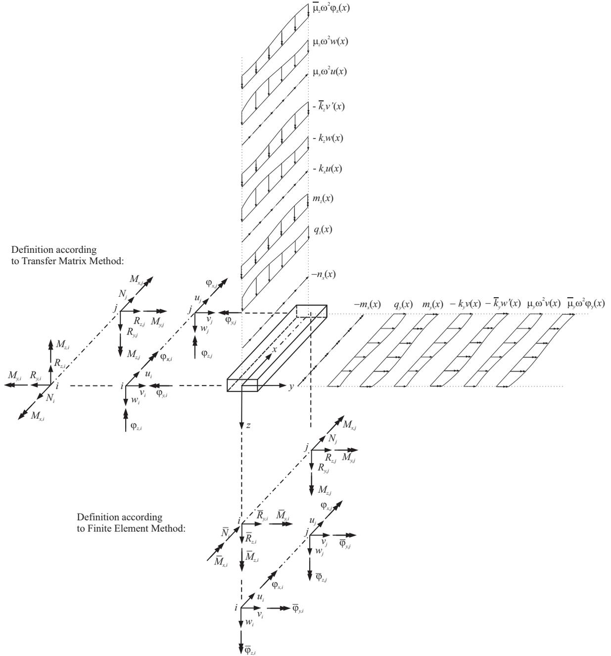
Figure 1: The local internal variables, static and inertia and loads for transfer matrix and finite element methods.
