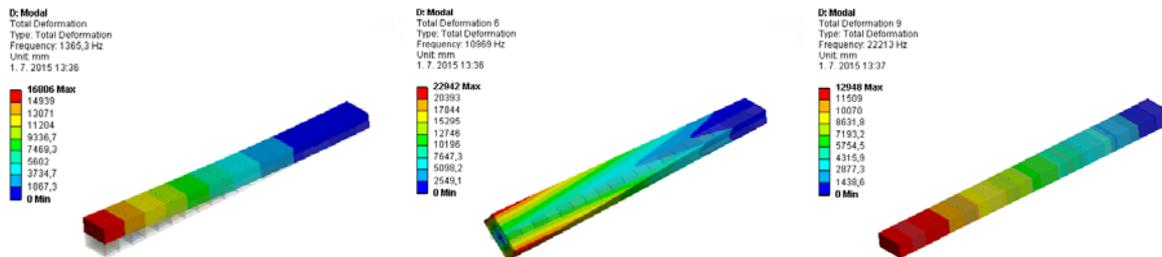
Figure 10: The 1<sup>st</sup> and 6<sup>th</sup> and 9<sup>th</sup> eigenforms of the beam (with Winkler elastic foundations).
