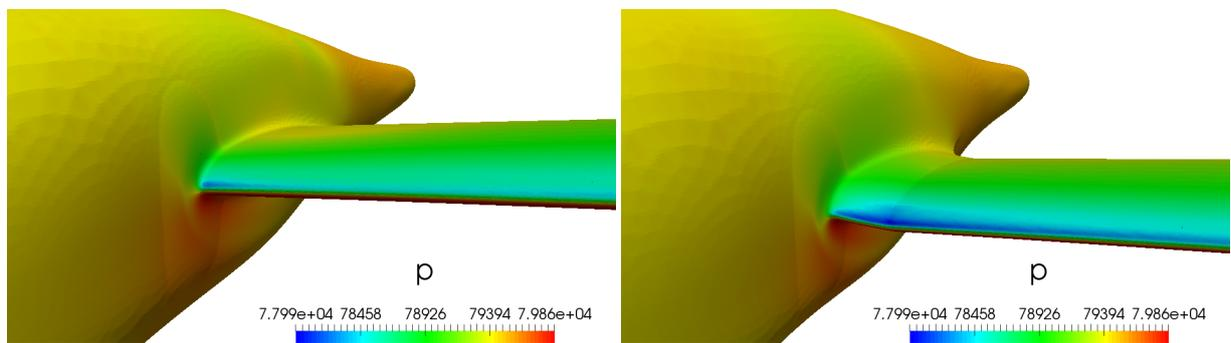
Figure 3: Optimization of an ultra-light aircraft. Comparison of the reference (left) and optimized (right) aircraft geometries. Close-up front view of the wing root-body junction.
