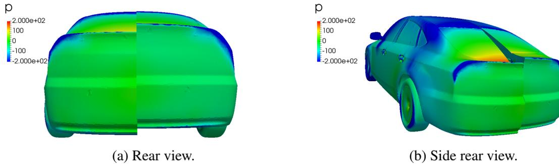
Figure 9: DrivAer car shape optimization. Comparison of the reference (right) and the optimized (left) car geometries.
