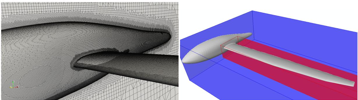
Figure 1: Optimization of an ultra-light aircraft. Close-up view of the wing root-body junction on a surface mesh (left) and RBF control boxes (right).
