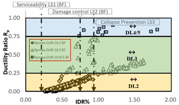
Figure 2: Comparison between the limit values IDR DL2-3-4 (V14) and LS1-LS2-LS3 (E08).
