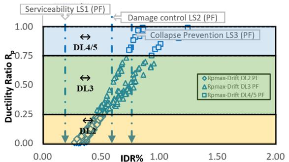
Figure 6: Comparison between the limit values IDR DL2-3-4 (V14) and LS1-LS2-LS3 (E08).
