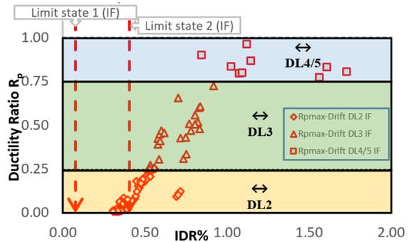
Figure 4: Comparison between the limit values IDR DL2-3-4 (V14) and LS1-LS2-LS3 (E08).
